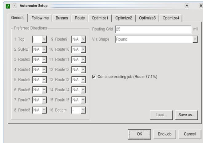
➤ *Autorouter setup: Restarting an interrupted job*
