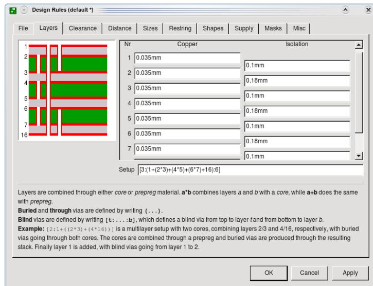
➤ Example 5: Layer Setup for an 8 layer board
