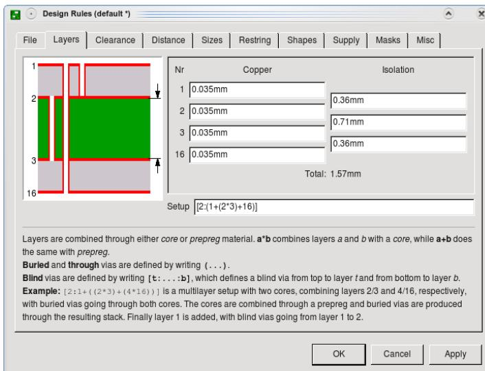
Layers are combined through either *core* or *prepreg* material.  $a*b$  combines layers *a* and *b* with a *core*, while  $a+b$  does the same with *prepreg*.
