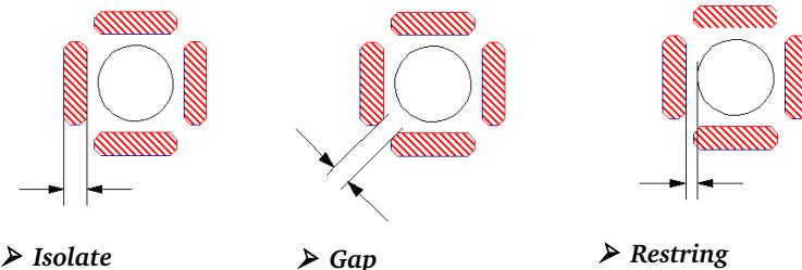
Pads or SMDs marked with the flag *NOTHERMALS* (CHANGE THERMALS OFF) in the Package Editor will be connected basically without Thermal symbols.
